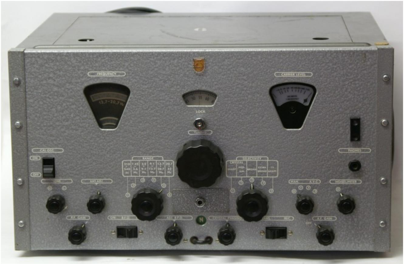
The Philips 635 receiver. This radio was used, primarily, to monitor the Greenwich time signals used for desert navigation. One wonders if the officers might not also have liked a bit of the symphony on the BBC, during afternoon tea!
