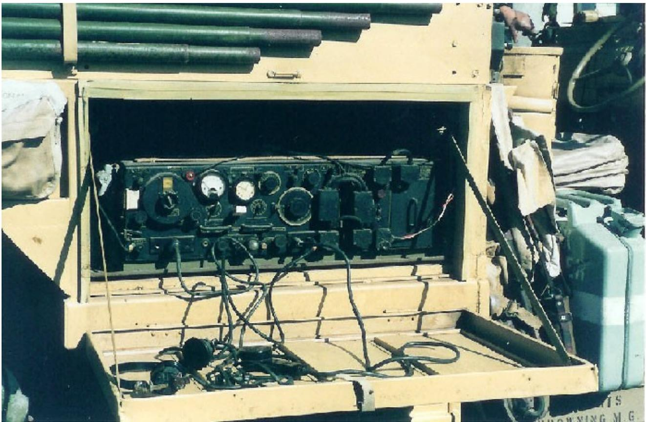
Wireless set No. 11, mounted in a 1 ½ ton Chevrolet truck. Note the right hand drive! Also note the headphones and straight key on the radio compartment door. There are also four 8 ½ foot poles mounted above the radio compartment. These were used to support the Windom antenna.
